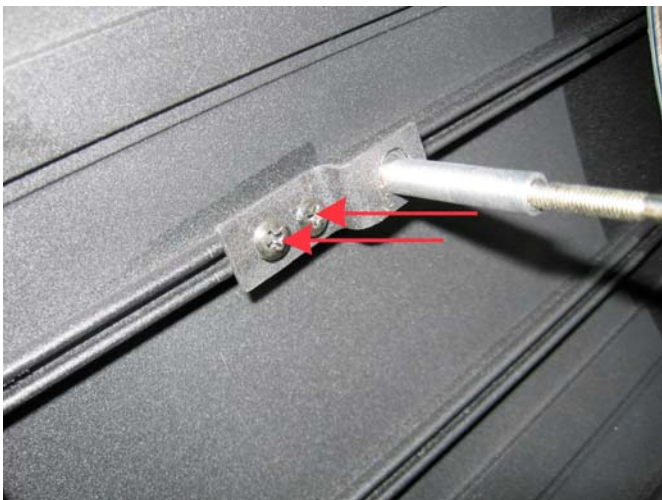
5. To remove the brackets, unscrew the 2 screws.
