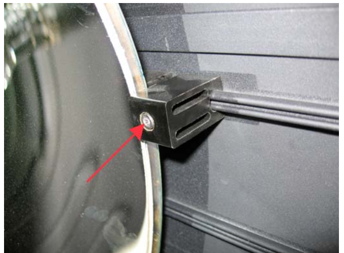
6. To remove the glass reflector unscrew this screw. Be very careful and try not to touch the glass. Do not bend or use force on the lamp, in this case the lamp can explode.
