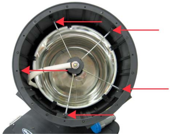
4. Remove all 5 lamp brackets
