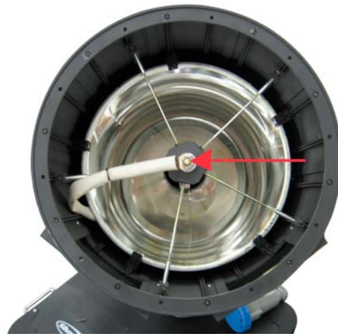
2. Remove the screw
