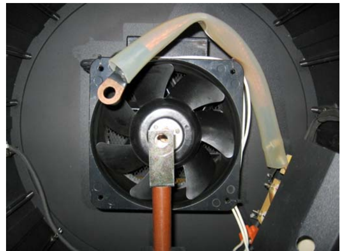
8. The screw on the backside of the lamp can now be removed and you can take out the lamp.
