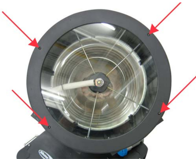
1. Remove the 4 screws
